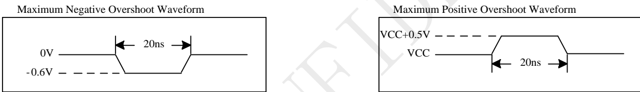
Figure 5-1 Maximum Overshoot Waveform
