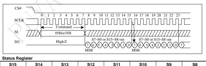
Figure 10-5 Read Status Register (RDSR) Sequence (Command 05 or 35)
