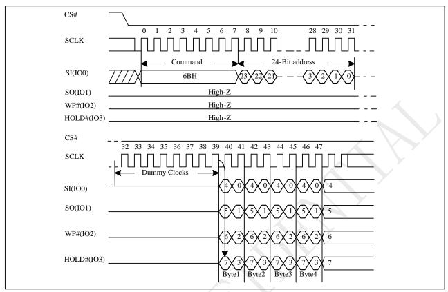
Figure 10-13 Quad Read Mode Sequence (Command 6B)
