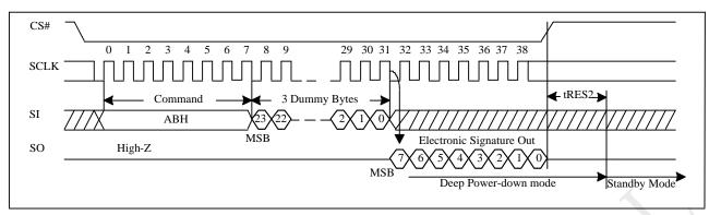
Figure 10-30 Release from Deep Power-down (RDP) Sequence (Command AB)
